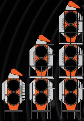
**CF2001 Configuration:** Single module, two fans & heaters, each with its own plenum in a 50/50 split.
