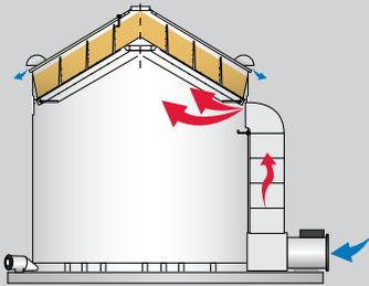
**Step 1.** One or two fan(s) and heater(s) force hot air through an even layer of wet grain in the drying chamber directly or through ductwork.
