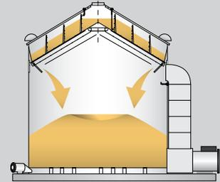
**Step 3.** When the grain has dried to a predetermined temperature, the actuator opens the dump chutes automatically, letting 1/4 of the hot dried grain in a 36', or 1/3 in the 24' or 30', fall into the cooling and storage area. The drying chamber is then automatically refilled, and the drying process continues until the grain supply is empty.
