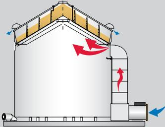
**Step 1.** One or two fan(s) and heater(s) force hot air through varied depth layers of wet grain in the drying chamber directly or through ductwork.
