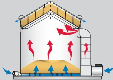
**Step 2.** Outside air from the cooling fan captures heat from previously dried grain and that heat and aeration air is used to help dry the next batch.
