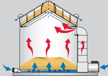
**Step 2.** Outside air from the cooling fan captures heat from previously dried grain and is then reused in the continuing drying process.
