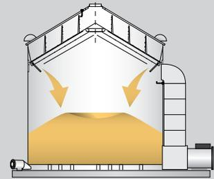
**Step 3.** When the column of grain has dried to a predetermined temperature, the fan(s) and heater(s) stop, and the operator manually opens the dump chutes letting the hot dried grain fall into the cooling and storage area below. The drying chamber is then manually refilled, and the operator can start the next batch drying.
